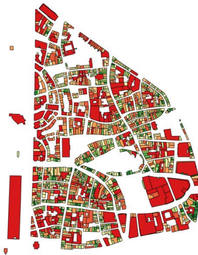
Figure 2: Example of Output of Bottom-Up H&C Demand Mapping Approach – Map View at Building Level
