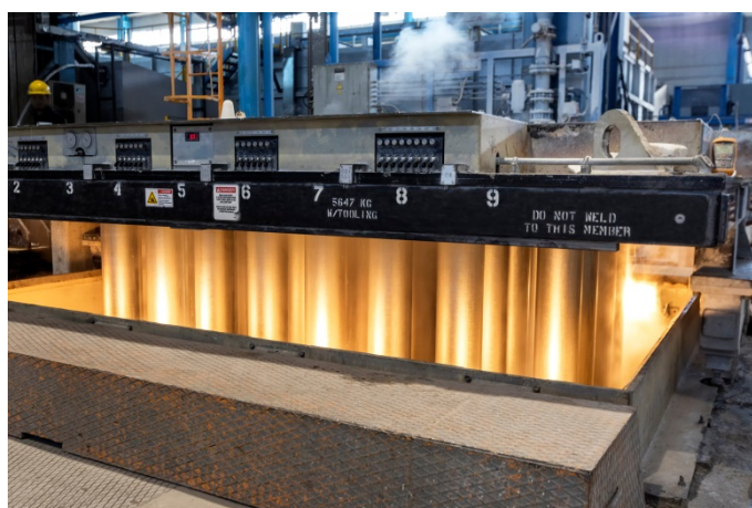
Figure 4: Electrolytic Hall-Héroult smelting process. Source: Shutterstock
